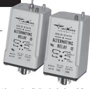
The Model 261 series Alternating Relay is designed for duplex pumping systems where it is desirable to equalize pump run time. The solid state alternating circuit drives an internal electromechanical relay. A continuous power source and control switch are required.
